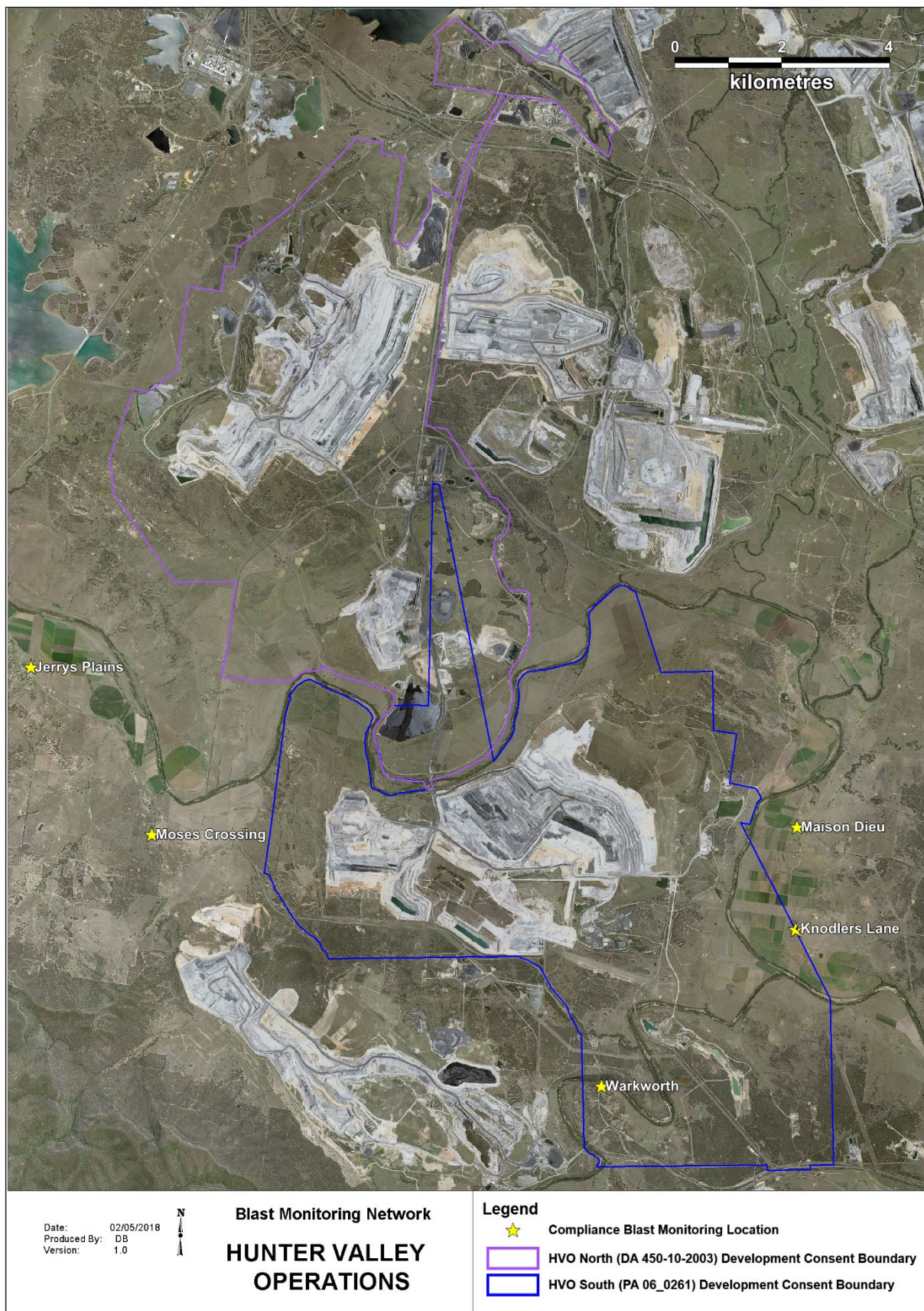
Figure 10: Blast Monitoring Location Plan
